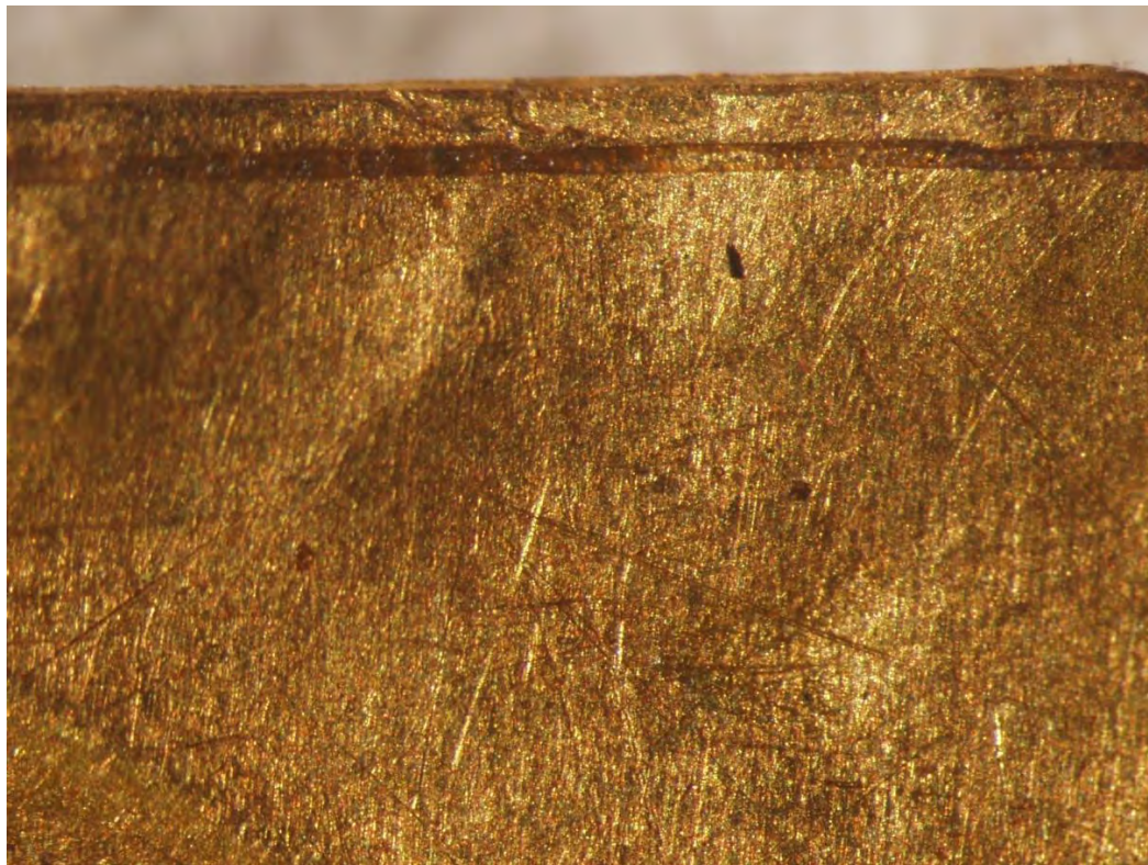
Photo #13: Thin groove along edge of back side of the lamella at 60X. (Wolter, 2017)
