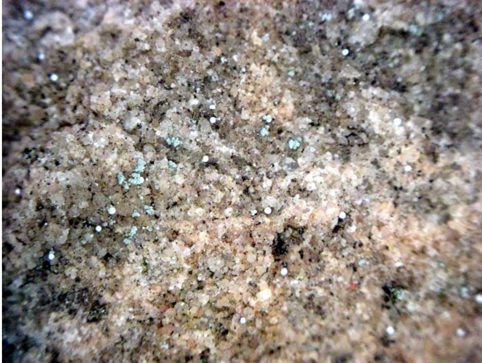
A close-up view of the Everson monument surface (87 years old) shows a less advanced weathering profile with a lesser amount of the loss of the clay cement between sand grains (15X).
