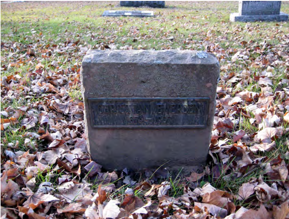
The Christian Everson monument in the Askov Cemetery is comprised of Hinckley Sandstone and having been erected in 1927 serves as a second excellent weathering control sample.
