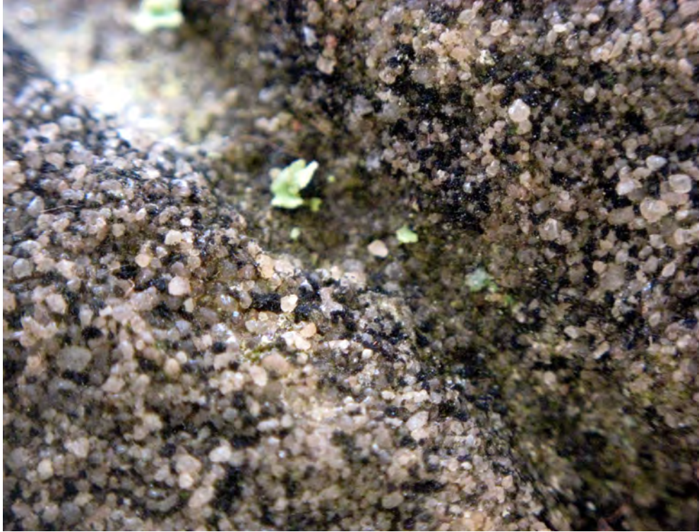
A close-up view of the groove in the number "1" shows significant rounding of the carved line and significant loss of the clay cement between sand grains consistent with advanced weathering (15X).
