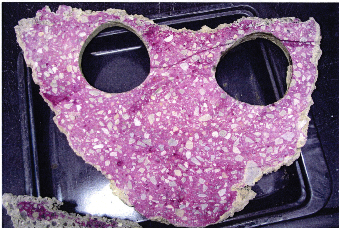
SAMPLE ID: P1-P2 DESCRIPTION: Carbonation (unstained) proceeds thinnly around the perimeter of the placement and leg impressions.
