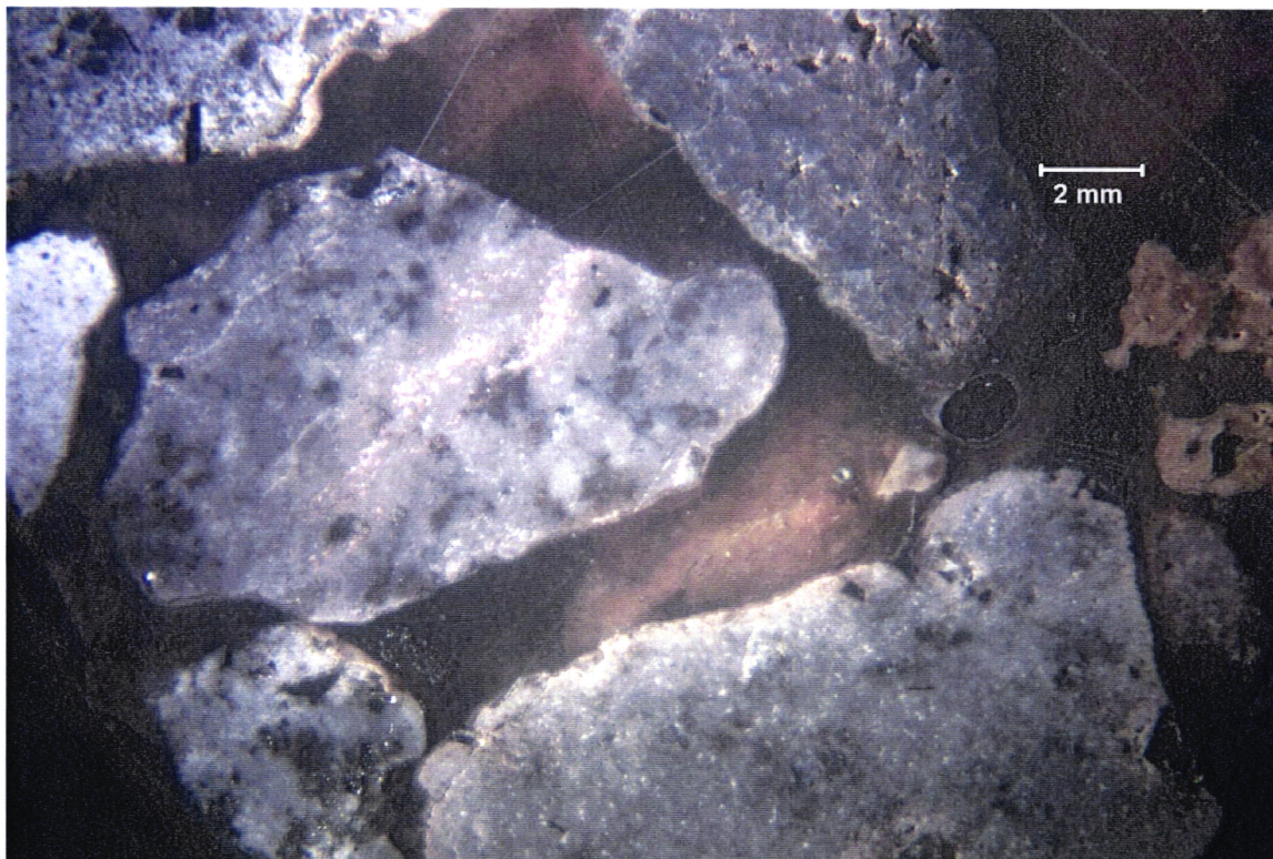
SAMPLE ID: Crime Scene Material DESCRIPTION: Overall view of the basalt aggregate in polished cross section of material retained on the #4 sieve. MAG: 7.5x
