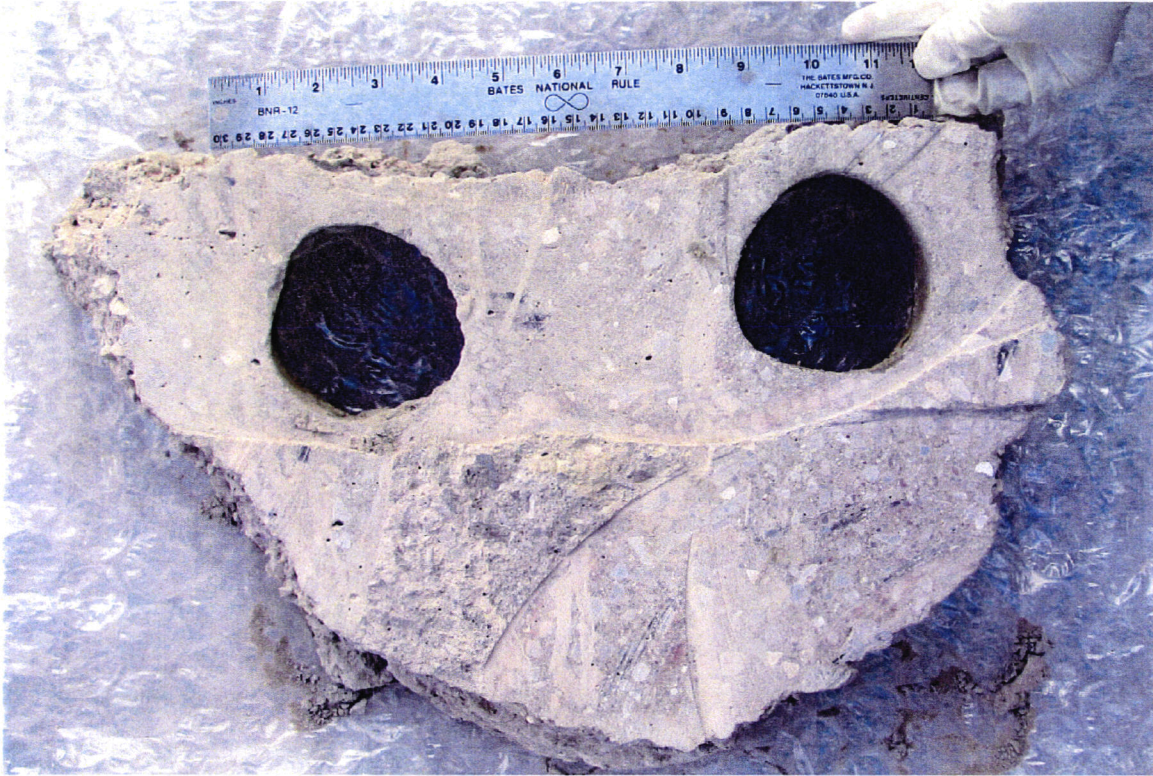
SAMPLE ID: P1-P2 DESCRIPTION: Sawcut section of concrete as recieved.
