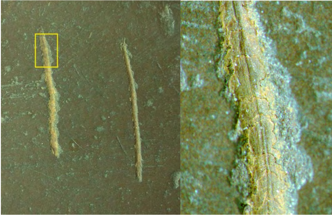
Figures 8 & 9: A closer view of the top portion of the scratched groove (character # 11) inside the yellow box shows iron-rich orange-colored clay that was produced when the instrument crushed the exterior weathering rind. The crack pattern in the clay-filled groove indicates the probe made the scratch in the direction of bottom to top (Right, 50X).
