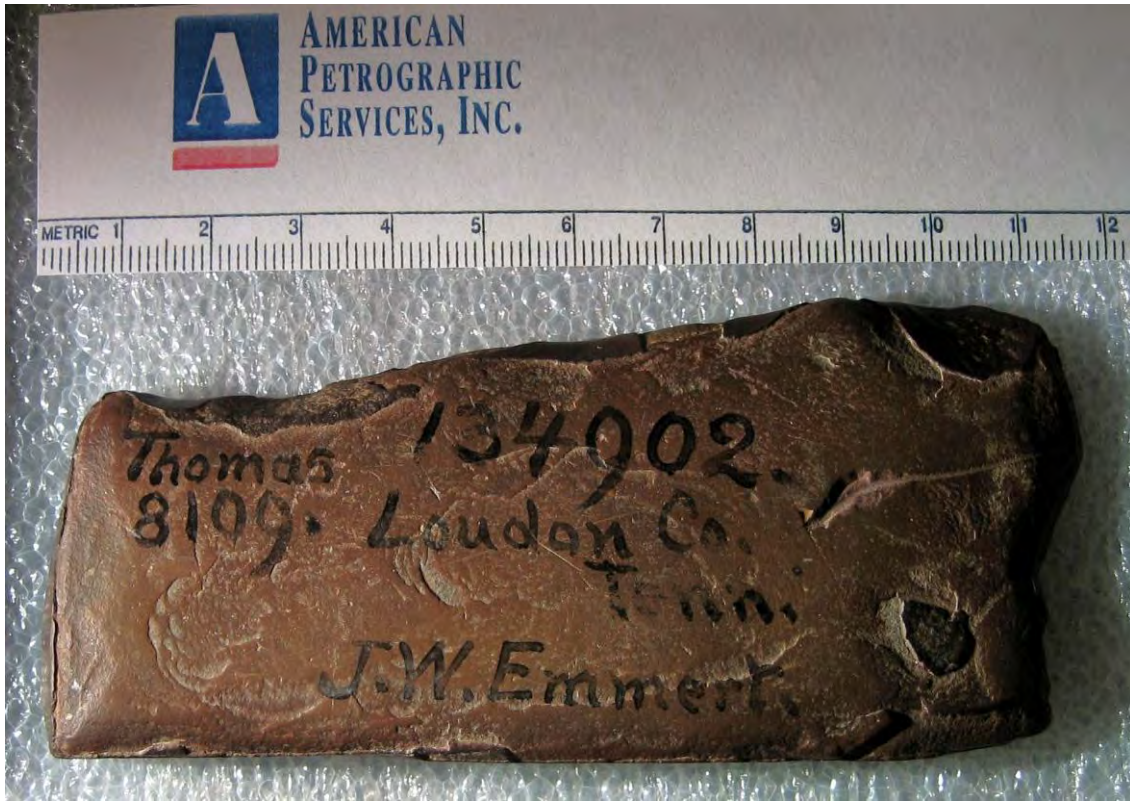
Figure 6: The back side of the Bat Creek Stone has the original Smithsonian (Institute) identification names and numbers. Virtually all but a few remnants along the top and bottom edges, and the small arrowhead-shaped portion on the lower right side, of the approximately 1-2 mm thick iron oxide-rich weathering rind has peeled off exposing the light brown-colored, unweathered iron-cemented clayey siltstone. The scratch made by Emmert with the metal prod at the time of the excavation is on the far right.
