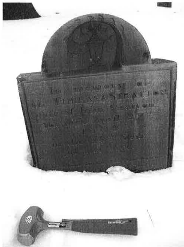
The Theresa Stratton tombstone (1802) and the equipment used in sampling. The climate in Hallowell, Maine is comparable to Kensington, Minnesota. Because of the snow and frozen ground only above grade samples were obtained.
