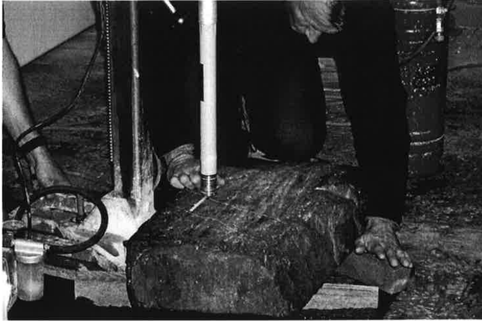
The 1-1/4" diameter diamond studded coring bit being positioned on October 3, 2000.
