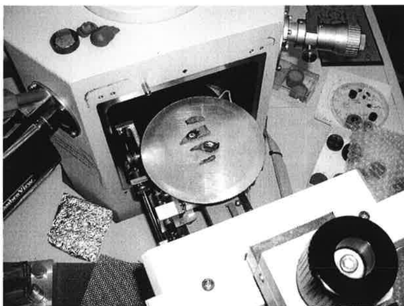
Tombstone chip samples #1, 2, 3 and 22 being loaded into the SEM sample chamber.
