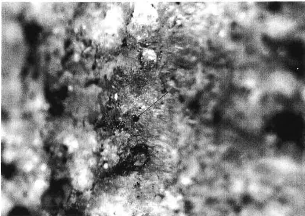
An actively corroding pyrite crystal (red arrow) creates a pronounced halo of iron oxide within a carved character on the AVM Stone (60x).
