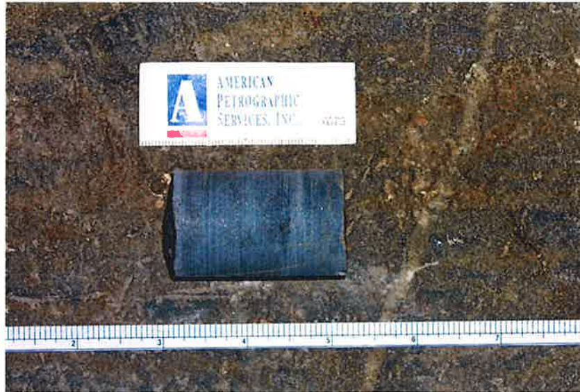
Figure #32: The 2" (50 mm) long sample after coring.
