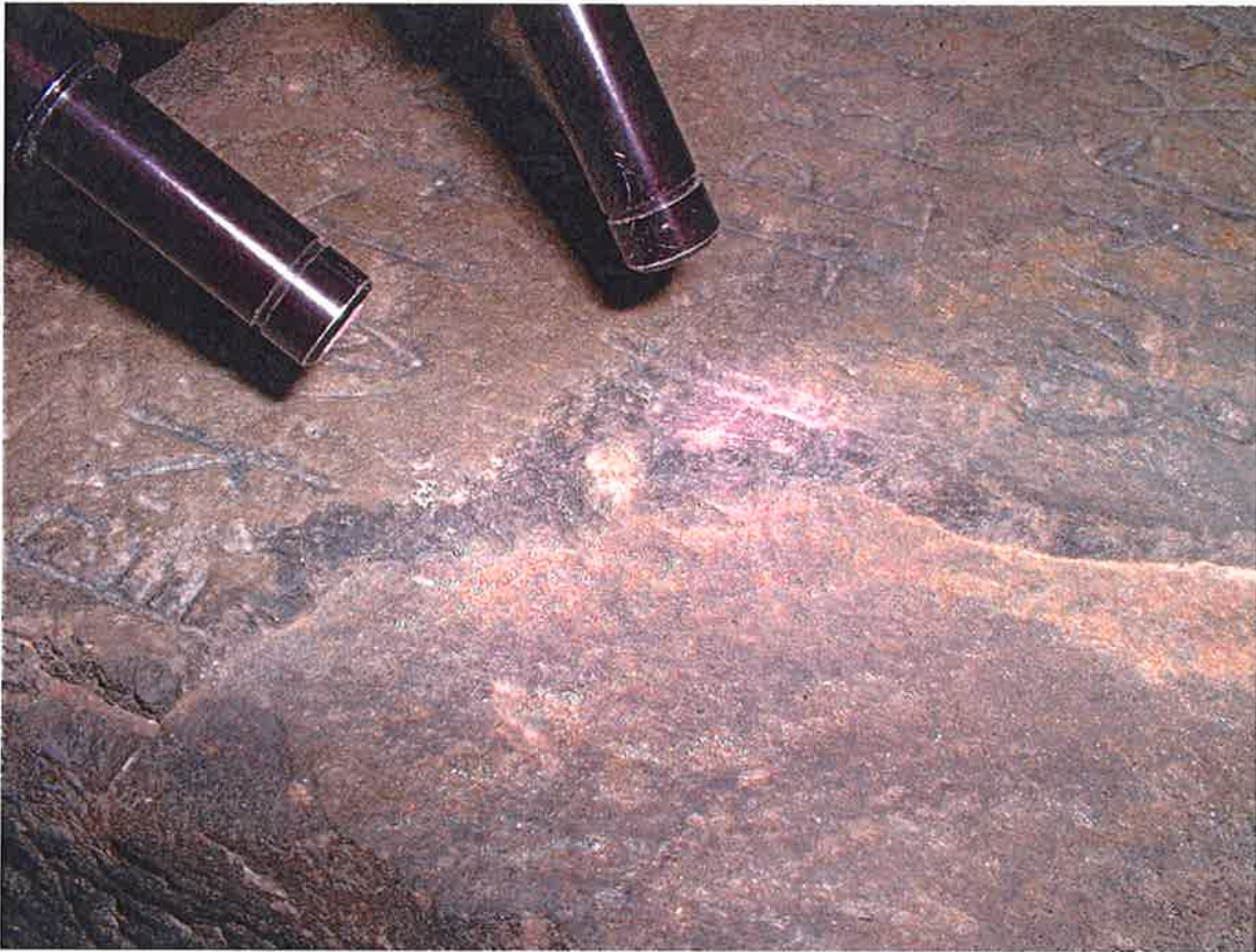
Figure #4: A relatively large piece of rock spalled off along the lower cleavage plane as the second line of the inscription was being carved.
