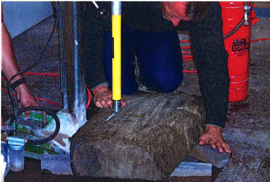
Figure #31: A 1 1/4" (32 mm) diameter diamond-studded coring bit is positioned over the backside of KRS.
