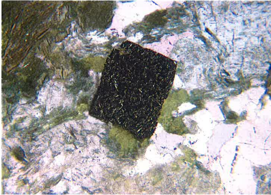
Figure #26: A pyrite crystal exhibiting cubic habit and a gold-colored metallic luster under plane polarized and reflected light, in a thin section made from the core sample obtained from the AVM Stone.
