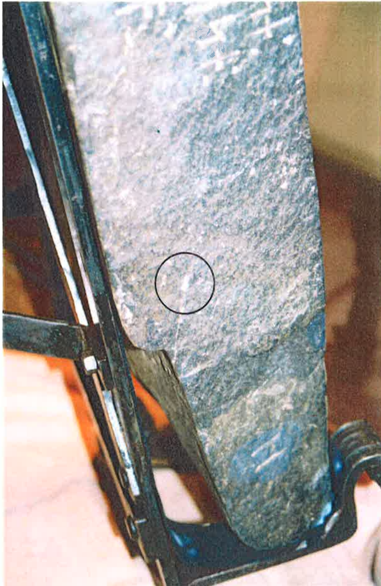
Figure #43: Location of the chip sample obtained from the split side.
