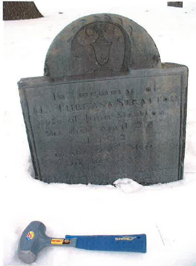
Figure #51: The Theresa Stratton tombstone (1802) and the equipment used in sampling. The climate in Hallowell, Maine is comparable to Kensington, Minnesota. Because of the snow and frozen ground, only above-grade samples were obtained.
