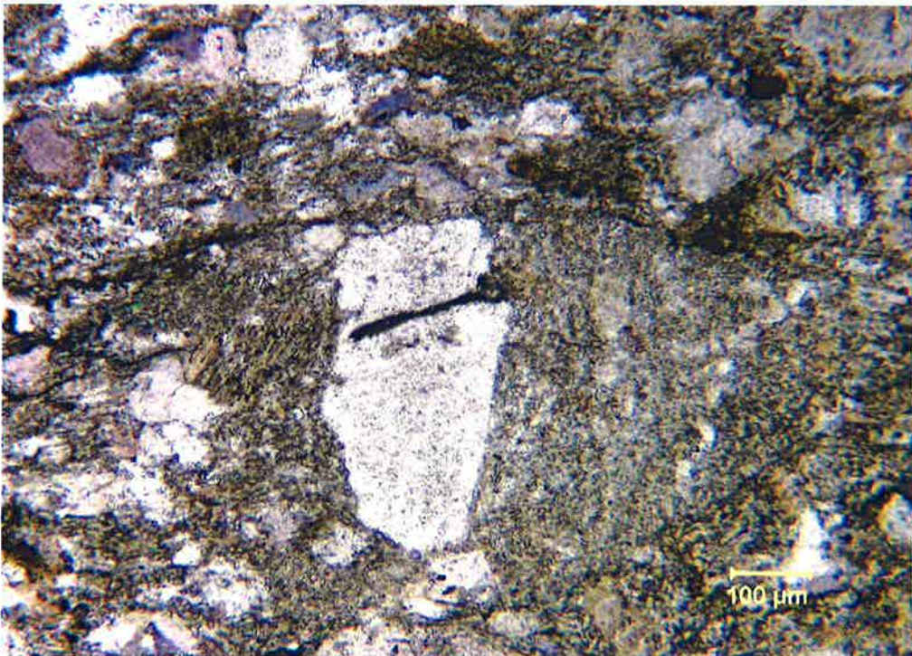
Figure #38: Rock fragments, like this porphyritic felsic volcanic clast under plane polarized light, comprise roughly 18% of the KRS.
