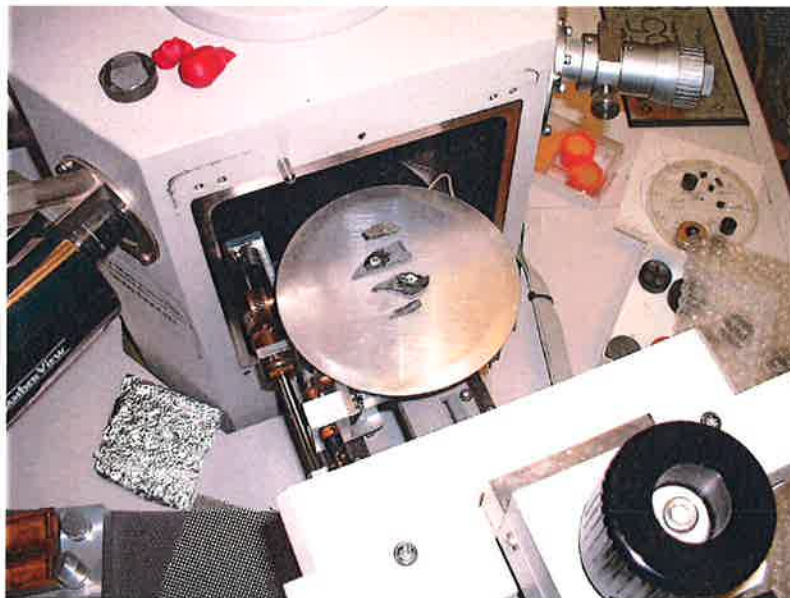
Figure #52: Tombstone chip samples being loaded into the SEM sample chamber.
